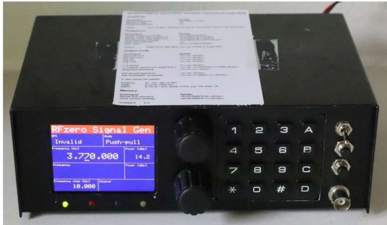
The RFzero signal generator with an ILI9341 2,8" display and keypad. Picture courtesy Hans, OZ2XH.
